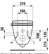
Connection with Laufen installation system INEOLINK
