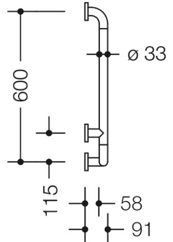
Abmessungen in mm
