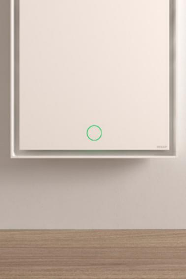
The **Irsap Temperature Regulator** is a device that permits the control of the FACE thanks to a pressure and rotation maneuver element. Luminous signals make maneuvers easy. Rotating the color interface adjustment dial permits the regulation of set-point temperature from a minimum 16°C to a maximum 26°C in 0.5°C steps. The summary table is provided below:
