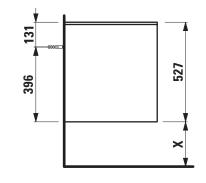
X = The exact height must be set during installation.
