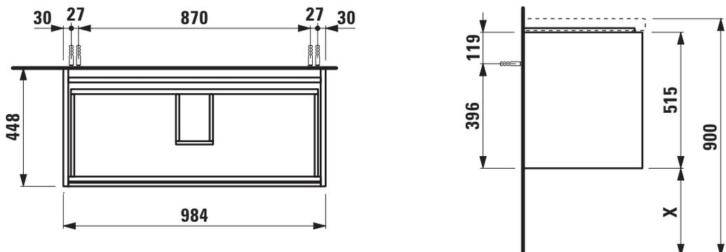
X = The exact height must be set during installation.
