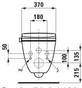
Connection with Laufen installation system INEOLINK
